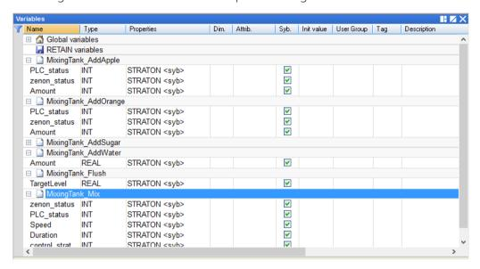
Mark the line **Properties** of the corresponding variable. Press **Ctrl+F12**. Thus the profile zenon Logic is displayed in this line. In addition you must activate the checkbox for embedding the symbol via double click or **Enter** in column **Symb**..
