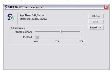
Depending on the size of the PLC application and the set cycle time, the slider has to be adjusted to the PLC load. The slider can be set between 10% and 85%. The current load is visualized as a bar and indicates whether the permitted maximum for executing the PLC cycle is sufficient.
